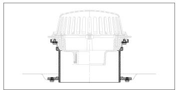
The -DR Top-Set Drain Riser Assembly is very similar to the -EA; however, the extension portion is completely removed from the path of the waterway.
