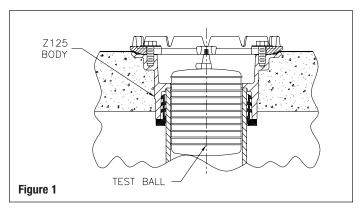
The Zurn Neo-Loc Gasket with Integral Test Cap eliminates the need for multiple test plugs and requires no loss of time for setup, prior to line system pressurization. The test cap is already in place when the drain body is installed, allowing for immediate testing (Figure 2). There is no need to carry multiple plugs from one drain fixture to another.
