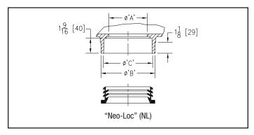
**Special Note:** Zurn "Neo-Loc" and "Sealtrol" gaskets are designed for use exclusively with Zurn drainage products. They are not sold separately and all warranties either expressed or implied would be forfeited if used in other than a Zurn drainage product.
