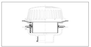
The -EA Adjustable Extension Assembly is very popular and often used when working with various degrees of roof insulation.
