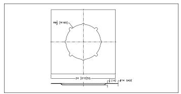
The roof sump receiver, also referred to as a bearing pan, is used when exact location of the drain can't be determined or when instances of opening the roof can not be precisely cut.
