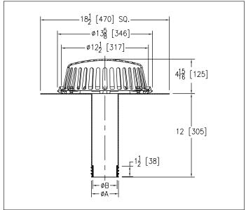
**RD2150-FS Flat Sump Replacement Roof Drain**
